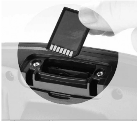
Inserting an MMC/SD into the Card Slot
