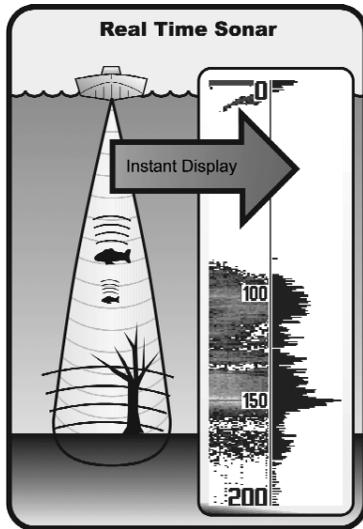
SONAR is an acronym for SOund and NAvigation Ranging. Sonar utilizes precision sound pulses or "pings" which are emitted into the water in a teardrop-shaped beam.
