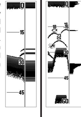
The **Wide RTS® Window** indicates the sonar intensity through the use of a bar graph. The length of the plotted return provides an indication of whether the return is weak or strong. The depth of the sonar return is indicated by the vertical placement of the return on the display depth scale.
