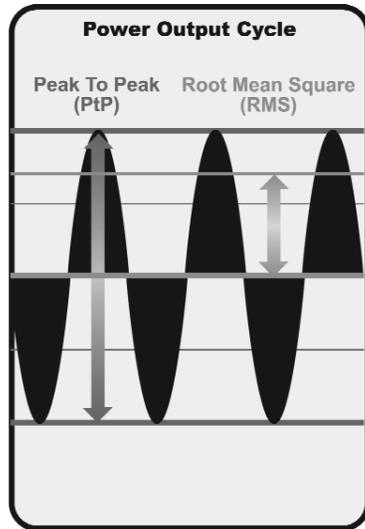
The power output is the amount of energy generated by the sonar transmitter. It is commonly measured using two methods:
