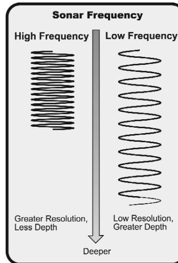
The sound pulses are transmitted at various frequencies depending on the application. Very high frequencies (455 kHz) are used for greatest definition but the operating depth is limited. High frequencies (200 kHz) are commonly used on consumer sonar and provide a good balance between depth. Low frequencies (83 kHz) are typically used to achieve greater depth capability.
