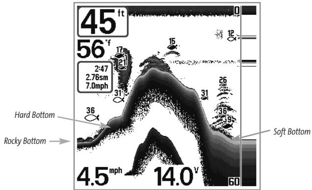
The sonar returns from the bottom, structure and fish can be represented as either **WhiteLine®** or **Structure ID®**. See *Sonar Menu Tab: Bottom View* for details on how to set the bottom view.
