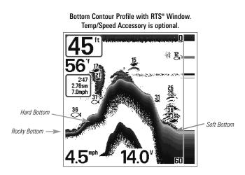
The sonar returns from the bottom, structure and fish can be represented as either Inverse (default), WhiteLine®, Structure ID®, or Bottom Black. See Sonar X-Press™ Menu: Bottom View for details on how to set the bottom view.
