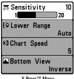
X-Press<sup>™</sup> Menu - The X-Press<sup>™</sup> menu allows you to access the settings that are changed frequently without having to navigate through the whole menu system. Press the MENU key once to display the X-Press<sup>™</sup> Menu. When you select a menu item from the X-Press™ menu. the menu will collapse, leaving only the menu choice on the screen. Use the UP or DOWN Cursor keys to reactivate the X-Press<sup>™</sup> menu.
