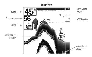
**NOTE:** If the Depth number is flashing, it means that the unit is having trouble locating the bottom. This usually happens if the water is too deep, the transducer is out of the water, the boat is moving too fast, or for any other reason that the unit can't accurately receive continuous data.
