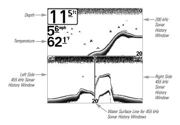
**Classic layout:** The top portion of the display presents a historical log of sonar returns from the 200 kHz down-looking sonar beam. The bottom portion of the display presents a historical log of sonar returns from the 455 kHz right- and left-looking sonar beams. New information appears at the top, and scrolls down the display.
