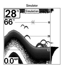
**NOTE:** To get the full benefit of the Simulator, it is important to select Simulator manually from the Start-Up Options menu as opposed to letting the Fishfinder enter Simulator automatically (as it will if a transducer is not connected and you do nothing during power up). Manually selecting Simulator from the Start-Up Options menu allows you to pre-configure your Fishfinder for on the water operation. Any menu changes you make will be saved for later use.
