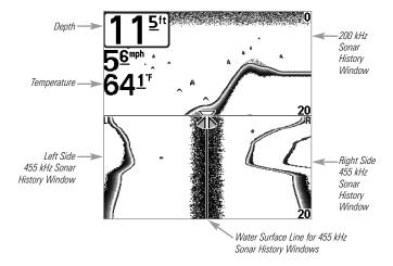
**Slanted layout:** This layout presents the two 455 kHz side sonar beams and the 200 kHz down-looking sonar beam as three panels of historical data. This layout is presented as three slanted panels. New information appears on the right, and scrolls to the left.
