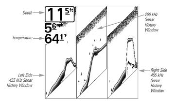
In all of these layouts, the sonar information from the side-looking beams reveals bottom contour, structure and fish similar to the down-looking beam, but the area covered is to the left and right of the area shown in the down-looking portion, so you actually see more of the bottom. The distance covered by the right and left beams is based on the depth setting for the down-looking beam, up to a maximum of 160 feet.
