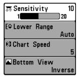
X-Press<sup>™</sup> Menu - The X-Press<sup>™</sup> Menu allows you to access the settings that are changed frequently without having to navigate through the whole menu system. Press the MENU key once to display the X-Press<sup>™</sup> Menu. When you select a menu item from the X-Press<sup>™</sup> Menu, the menu will collapse, leaving only the menu choice on the screen. Use the UP or DOWN Cursor keys to reactivate the X-Press<sup>™</sup> Menu.
