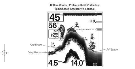
The sonar returns from the bottom, structure and fish can be represented as either **Inverse** (default), **WhiteLine®**, **Structure ID®**, or **Bottom Black**. See *Sonar X-Press*<sup>TM</sup> *Menu: Bottom View* for details on how to set the bottom view.
