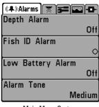
Main Menu System Normal User Mode **Main Menu Tabs** - Less frequently-adjusted menus are grouped into the Main Menu System. The Main Menu system is organized under the following tab headings to help you find a specific menu item quickly: Alarms, Sonar, Setup, Views, and Accessories.
