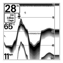
**Bottom Black** displays all pixels below the bottom contour as black, regardless of signal strength. This has the benefit of providing a high contrast between the bottom and other sonar returns on the display. Any targets such as fish, structure and thermoclines will be shown using the Structure ID<sup>®</sup> method.
