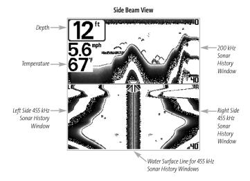
The sonar information from the side-looking beams reveals bottom contour, structure and fish similar to the down-looking beam, but the area covered is to the left and right of the area shown in the down-looking portion, so you actually see more of the bottom. The distance covered by the right and left 90° beams is based on the depth setting for the down-looking beam, up to a maximum of 160 feet.
