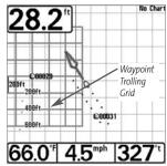
Add or Remove a Trolling Grid: From the Waypoints submenu, select Grid and press the RIGHT Cursor key to display a list of waypoints. Select the waypoint to which you want to add the grid. The trolling grid will appear on all of the navigation views, and can be used as a guide when trolling around a waypoint. The grid can be rotated to any desired heading using Grid Rotation from the Navigation Main menu. To remove the trolling grid, choose Remove Grid from the Navigation X-Press™ menu.
