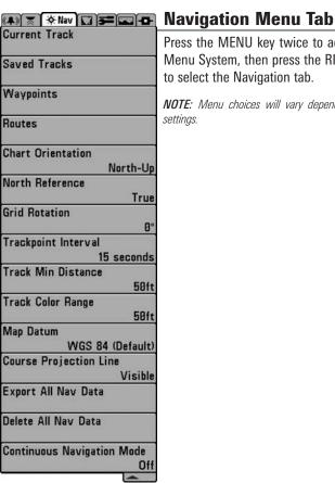
Press the MENU key twice to access the Main Menu System, then press the RIGHT cursor key to select the Navigation tab.
