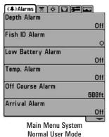
Main Menu Tabs - Less frequently-adjusted menus are grouped into the Main Menu System. The Main Menu system is organized under the following tab headings to help you find a specific menu item quickly: Alarms, Sonar, Navigation, Chart, Setup, Views and Accessories.
