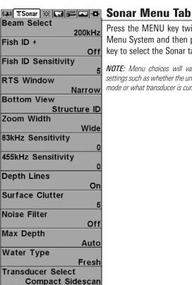
Press the MENU key twice to access the Main Menu System and then press the RIGHT Cursor key to select the Sonar tab.
