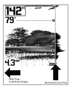
When all the echoes are viewed side by side, an easy to interpret "graph" of the bottom, fish and structure appears.
