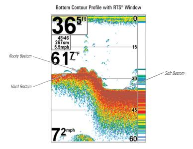
The sonar returns from the bottom, structure and fish can be represented as either **WhiteLine®** or **Structure ID®**. See *Sonar Menu Tab: Bottom View* for details on how to set the bottom view.
