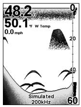
Sonar Page with Overlay Data turned on. This example shows Depth, Water Temperature and Water Speed.
