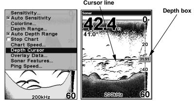
At left, Sonar Page menu with Depth Cursor command selected. At right, sonar chart with the depth cursor active. The school of fish is 31.91 feet deep.
