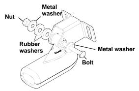
Assemble transducer and bracket.
