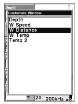
Water Distance has been picked to replace Water Temperature in the top digital data box.
