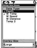
Overlay Data command on the Sonar Menu, at left. Overlay Data Shown selection menu, right. In this example, Depth will be displayed in a large font.
