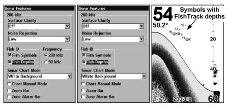
Sonar Features menu with Fish I.D. Depths selected (at left, dual-frequency menu; center, single-frequency menu). When the check box to the left is checked, the feature is on. At right, Sonar Page showing Fish I.D. symbols and FishTrack depths turned on.
