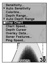
Sonar Menu with Stop Chart command selected. The box is unchecked, indicating that the chart is scrolling across the screen.
