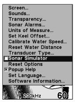
Main Menu with Sonar Simulator command selected. The Simulator is turned off (check box is unchecked).
