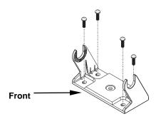
Install the gimbal bracket. Orient the bracket so the arms slope toward the front of your unit.
