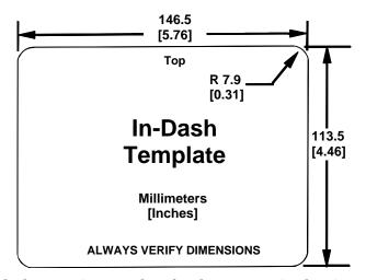
In-dash mounting template for the sonar unit, showing dimensions. NOTE: The figure above is *not* printed to scale. A scaled template (FM-5 In-Dash Adapter Kit instructions) is available for free download from our web site, www.eaglesonar.com.
