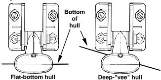
Align transducer centerline with hull bottom and attach transducer to transom. Rear view of dual-frequency Skimmer shown.
