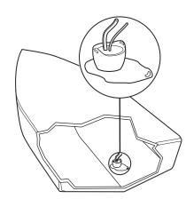
In-Hull Transducer with External Temperature Probe
