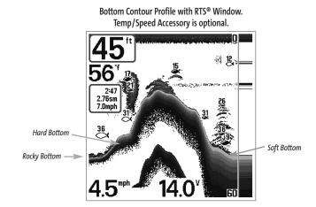
The sonar returns from the bottom, structure and fish can be represented as either Inverse (default), WhiteLine®, Structure ID®, or Bottom Black. See Sonar X-Press™ Menu: Bottom View for details on how to set the bottom view.
