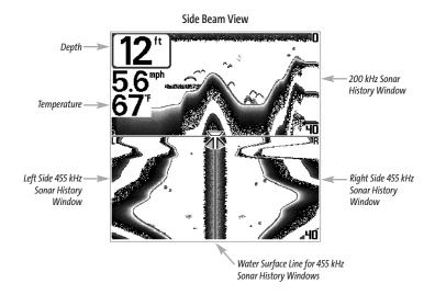
The digital readouts in the Side Beam View cannot be customized.
