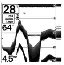
**Inverse** is a method where weak returns are shown with dark pixels and strong returns with lighter pixels. This has the benefit of ensuring that weak signals will be clearly visible on the display.
