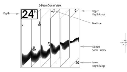
The digital readouts in the 6-Beam Sonar View cannot be customized, making information such as water temperature and voltage unavailable in this view.
