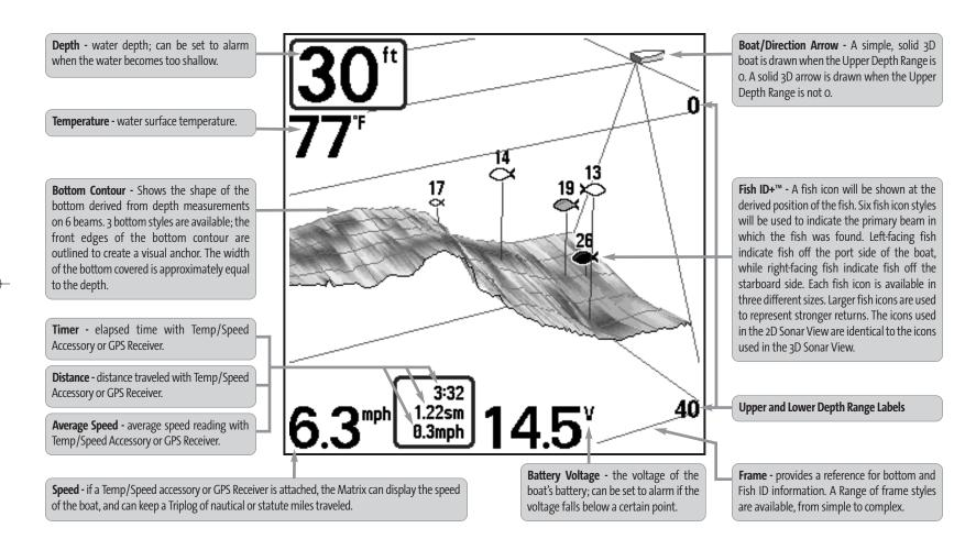
**NOTE**: Entries in this view that list (with Temp/Speed or GPS Receiver) are available if either device is the GPS receiver will be displayed on the view.
