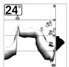
**Inverse** is a method where weak returns are shown with dark pixels and strong returns with lighter pixels. This has the benefit of ensuring that weak signals will be clearly visible on the display.
