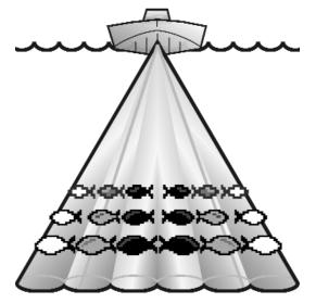
When Fish  $\mathsf{ID}+^{\mathsf{m}}$  is turned off, the Fishing System shows only the raw sonar returns on the display.
